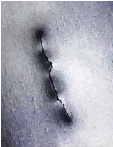
Fig. 5. Al 0.013 mm, crack detail.
