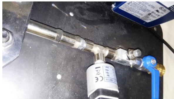
Fig. 3. Pressure piping system.
