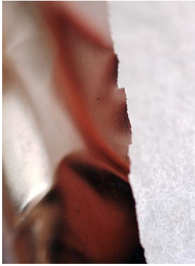
Fig. 12. FeNi alloy 0.05mm, crack detail.
