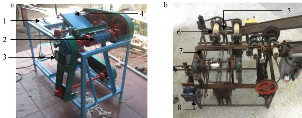
Fig. 2. (a) a carding machine; (b) a twisting machine.
