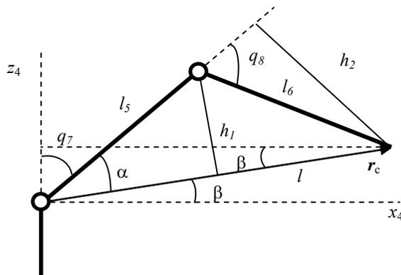
Fig. 2. The scheme for decision ITK of manipulator.
