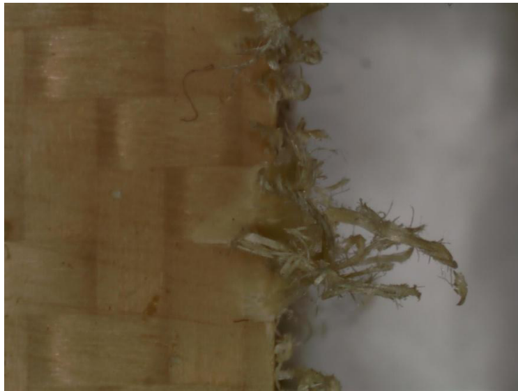
Fig. 2. Photograph of a frayed cutting edge after milling of an aramid fibre epoxy compound.
