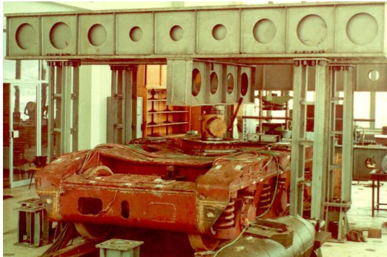
Fig. 1. Test setup of the bogie frame.
