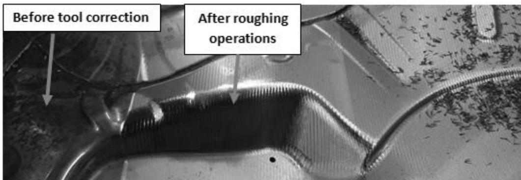
Fig. 6. tool paths (sweeping strategy method) after roughing of real workpiece in the CNC machine tool MECOF.
