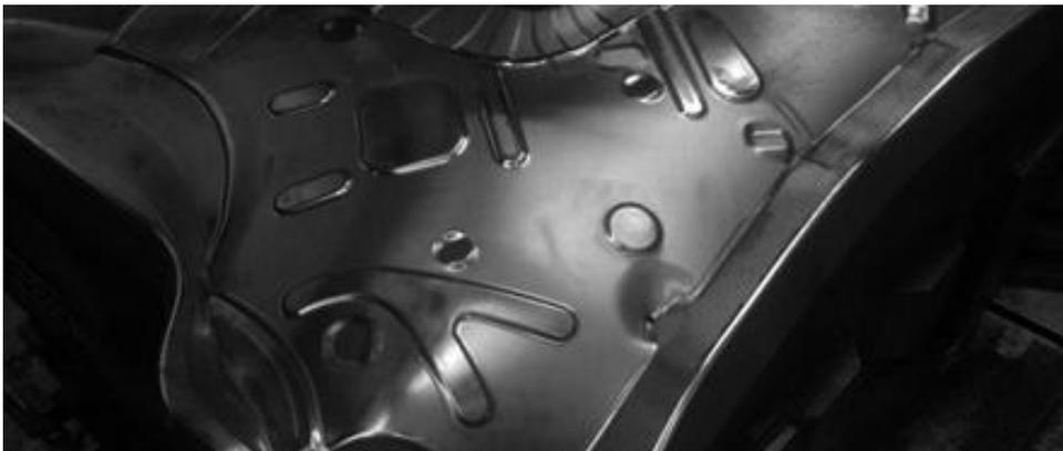
Fig. 12. machined surface with 8mm spherical milling cutter in the CNC machine tool MECOF.
