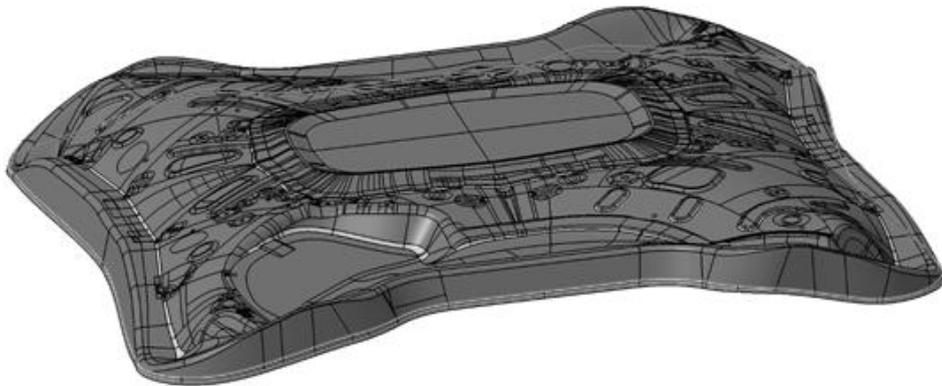
Fig. 2. the three dimensional surface C1 created in the CAD/CAM system CATIA V5 R20.
