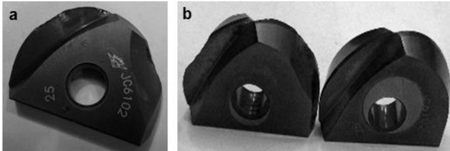
Fig. 13. (a) wear changeable wear cutting insert; (b) comparison of the new (right view) and wear (left view) insert.
