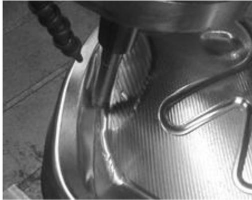
Fig. 10. an overview of the machined surface with 20 mm milling cutter in the CNC machine tool MECOF.
