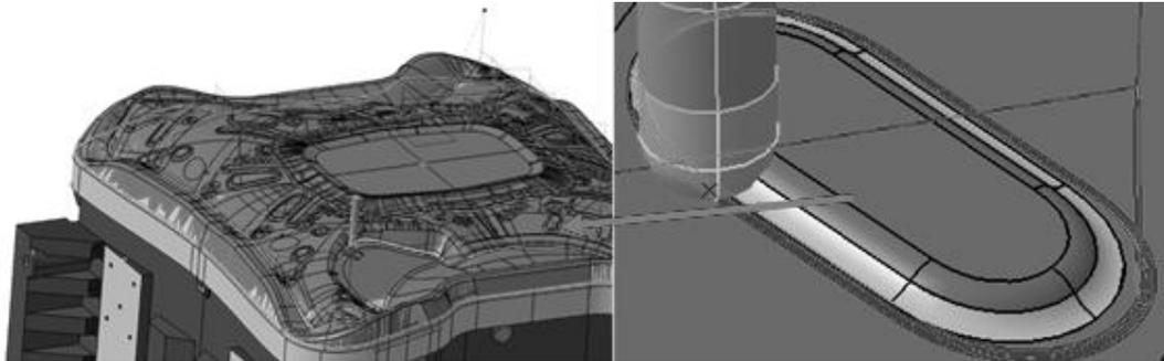
Fig. 7. tool path simulation of finishing strategy with 16 mm milling cutter machining in the CAD/CAM system CATIA.
