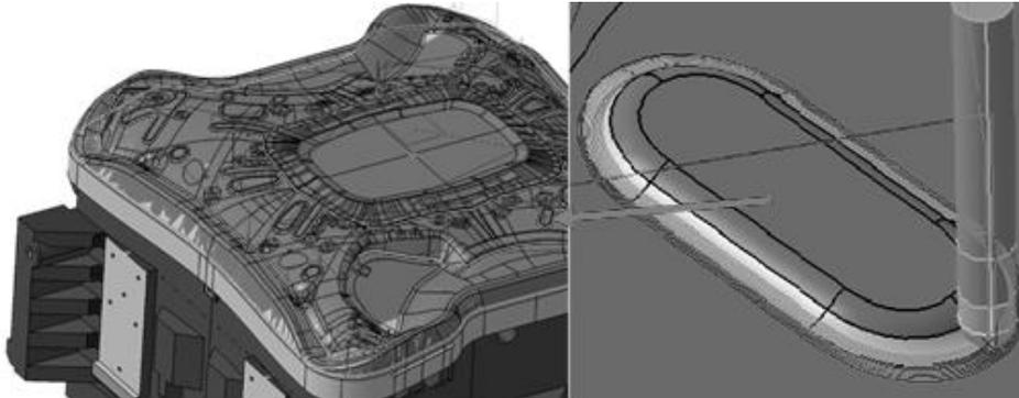
Fig. 11. tool paths simulation of finishing technology with 8 mm milling cutter in the CAD/CAM system CATIA.
