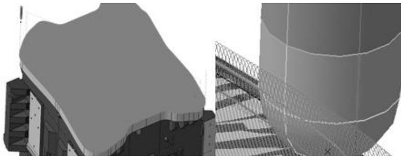
Fig. 9. strategy simulation of sweeping method with 20 mm milling cutter in the CAD/CAM system CATIA.
