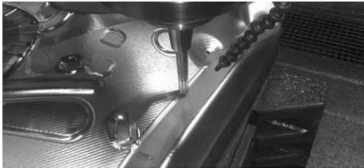
Fig. 8. tool paths of 16 mm spherical milling cutter during surface finishing in the CNC machine tool MECOF.
