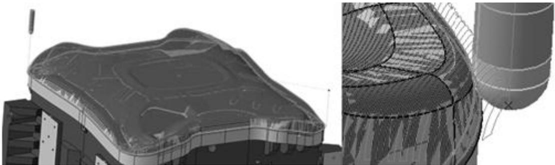
Fig. 5. milling cutter tool path strategy of roughing operation in the CAD/CAM system CATIA V5 R20.
