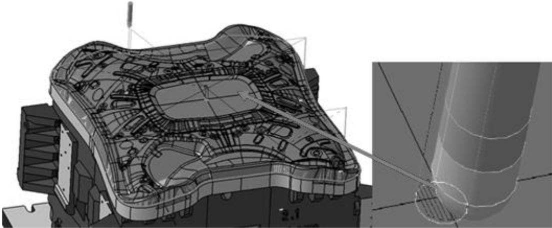
Fig. 4. simulation process of tool path of control milling in the CAD/CAM system CATIA V5 R20.
