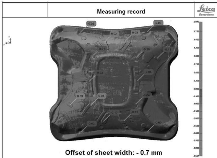
Fig. 14. view of the measuring report of scanned workpiece in the the Leica LTD840 T-Scan scanner.
