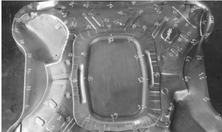
Fig. 1. the measured values of HRC hardness after surface hardening of workpiece by the flame.
