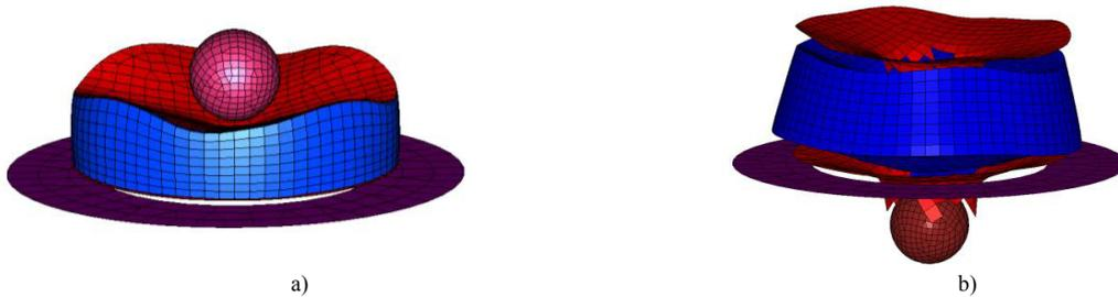
Fig. 10. Deformed shapes of two expanded polystyrene foam sandwich specimens a) with steel layers; b) with aluminium layers.
