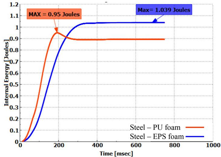
Fig. 14. Time dependence of the absorbed energy for the steel layered polyurethane/ expanded polystyrene sandwich structure.
