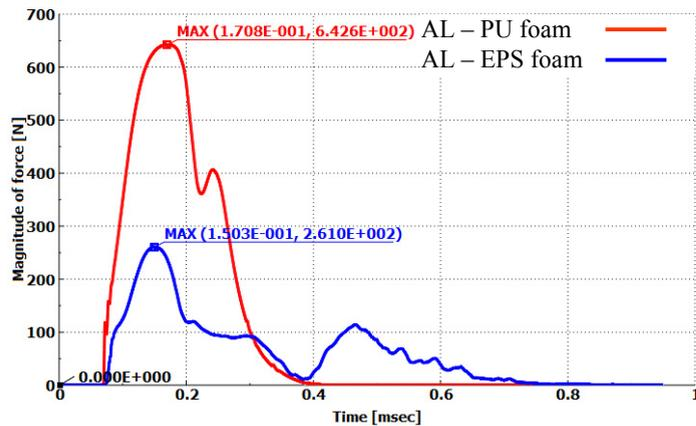
Fig. 13. Time dependence of the contact force intensity between the aluminium layered polyurethane/ expanded polystyrene sandwich structure and the support.
