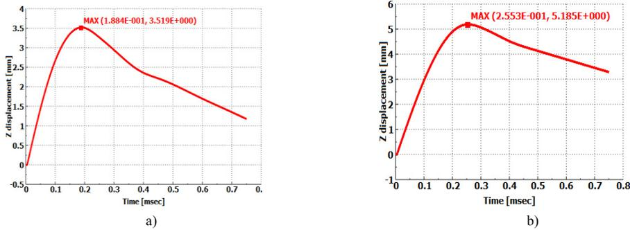
Fig. 9. Displacement – time variation for steel (a) and aluminium (b) sandwich configurations.
