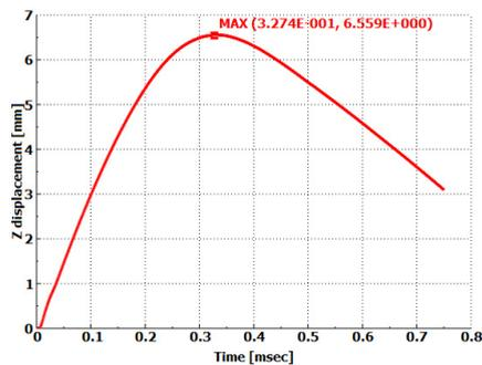
Fig. 5. Time-displacement variation for the PU foam without metallic layers.
