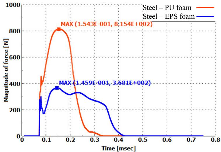
Fig. 12. Time dependence of the contact force intensity between the steel layered polyurethane/ expanded polystyrene sandwich structure and the support.
