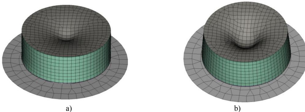
Fig. 8. Deformed shapes of two polyurethane foam sandwich specimens
