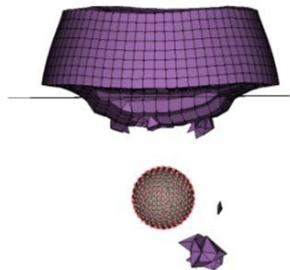
Fig. 6. Perforation of polystyrene specimen.
