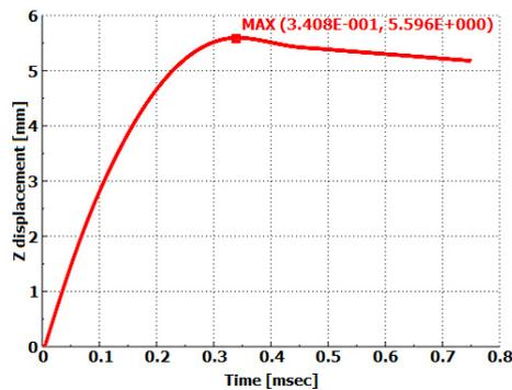
Fig. 11. Displacement – time variation for steel expanded polystyrene foam sandwich configuration.
