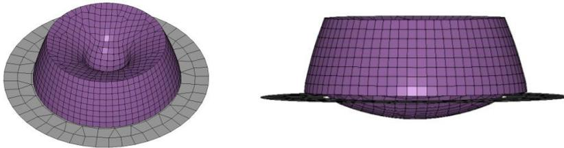
Fig. 7. Deformed shape of polyurethane foam specimen.
