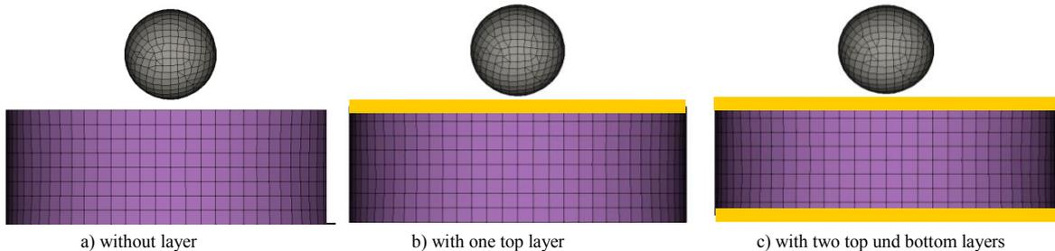
Fig. 3. Configurations of impact tests.
