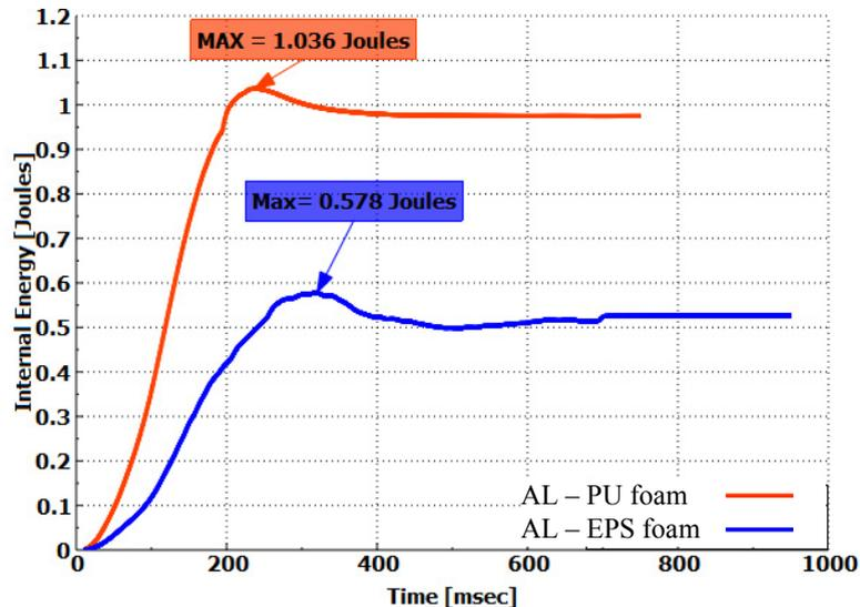
Fig. 15. Time dependence of the absorbed energy for the aluminium layered polyurethane/ expanded polystyrene sandwich structure.
