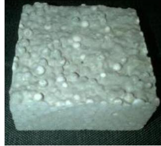
Fig. 2. Expanded polystyrene foam specimen.
