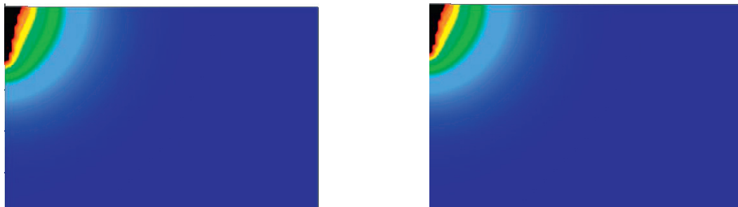
Fig. 6. Temperature distribution at different time steps: 0.2 ms (left) and 0.05 ms (right).
