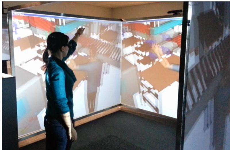
Fig. 6. Placement of components in the workplace using the CAVE.
