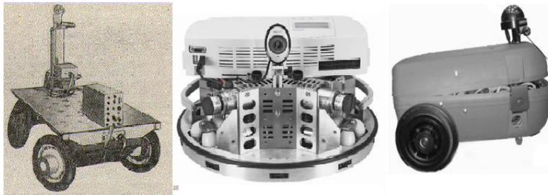
Fig. 1. One of our first (1985) educational mobile robots with scanning ultrasonic locator and controlled by PC with microprocessor (left photo). Configuration of modern educational mobile robots: Robotino (designed by “Festo”) and AMUR (right, designed by “Sensorika” Laboratory, KIAM RAS) within the virtual laboratory “Intelligent Robotronics”.
