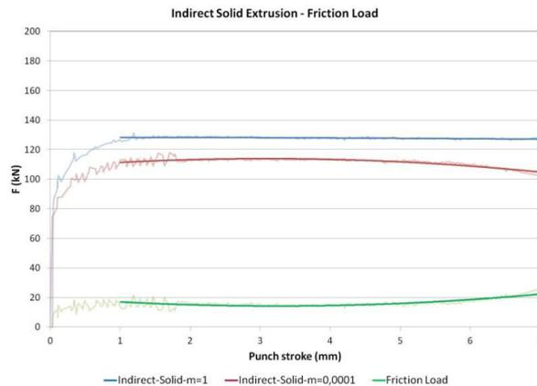
Fig. 7. Friction load for indirect solid extrusion.
