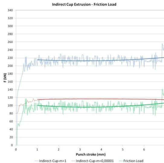
Fig. 9. Friction load for indirect cup extrusion.
