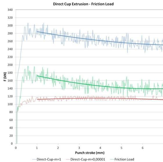
Fig. 8. Friction load for direct cup extrusion.
