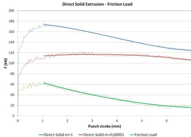
Fig. 6. Friction load for direct solid extrusion.
