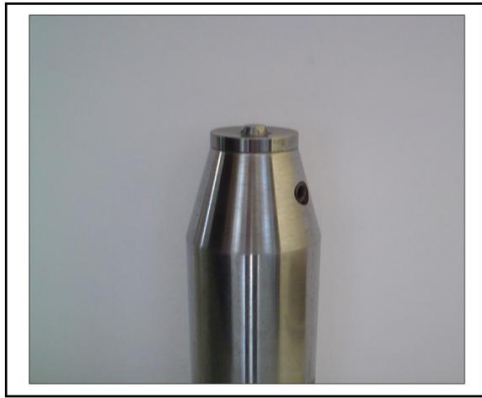
Fig. 3. Tool 3 geometry: carbide tool large shoulder.
