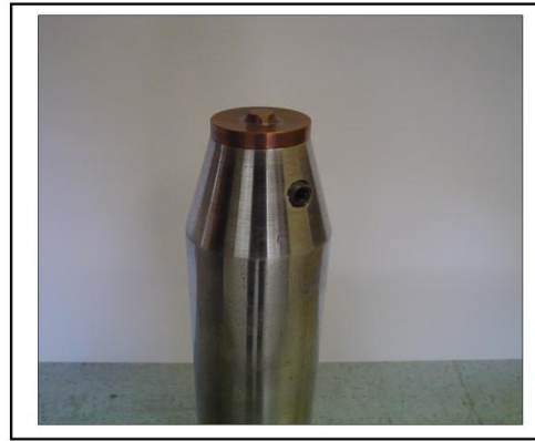
Fig. 4. Tool 4 geometry: carbide tool large shoulder with coating.
