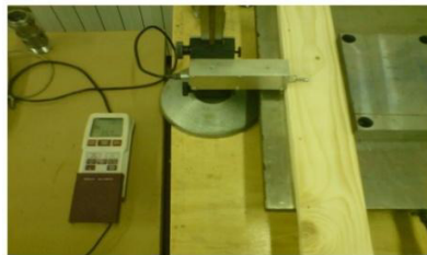
Fig 7. Measurement of surface roughness using a device Mitutoyo SJ-201.
