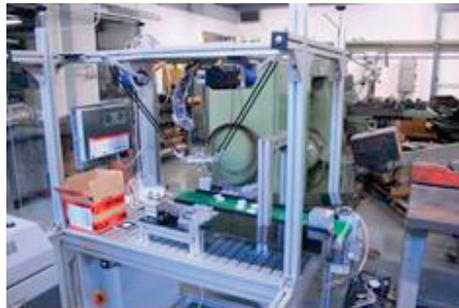
Fig.3. Sorting workplace with delta robot.
