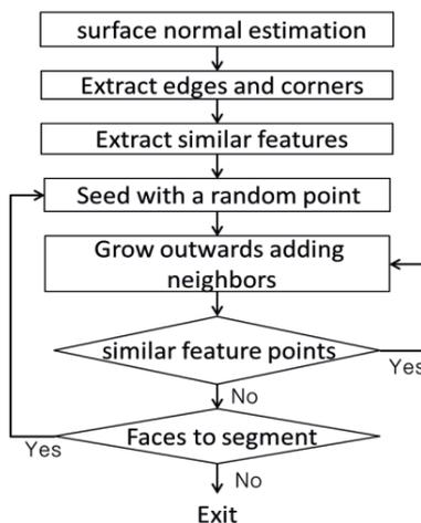
Fig. 2. Schematic representation of region growing segmentation algorithm.
