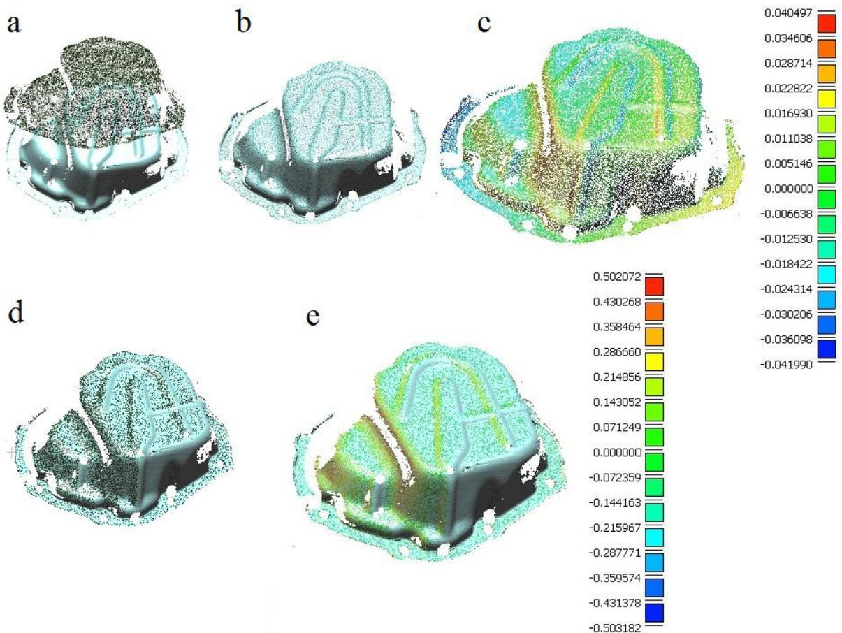
Fig. 4. (a) initial position of two patches (b) position after registration (c) visualization of error distance between registered patches (d) Registration with point to point ICP algorithm(Besl and Mckay method).
