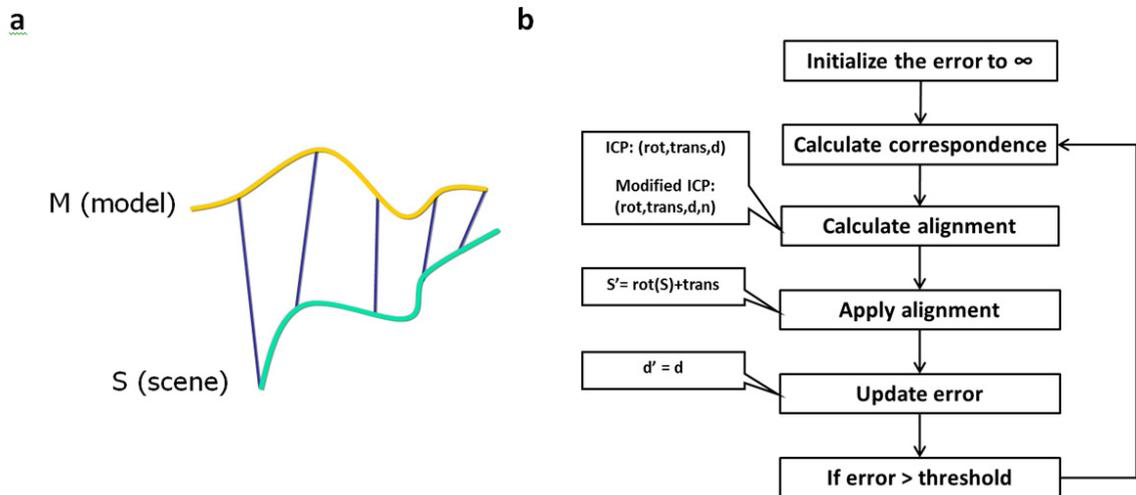
Fig. 3. (a) Illustration of registration process using ICP algorithm (b) Schematic representation of registration algorithm.
