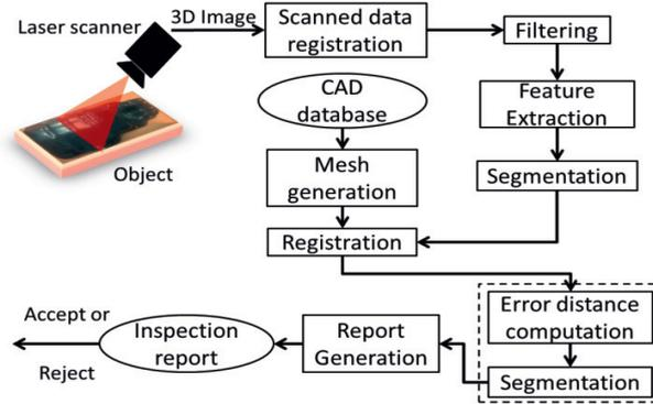
Fig. 1. Schematic procedure to represent the inspection system. [1]
