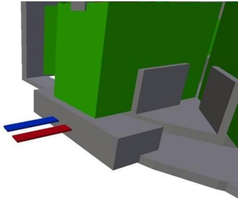
Fig. 12. Contact pins on the swapping station
