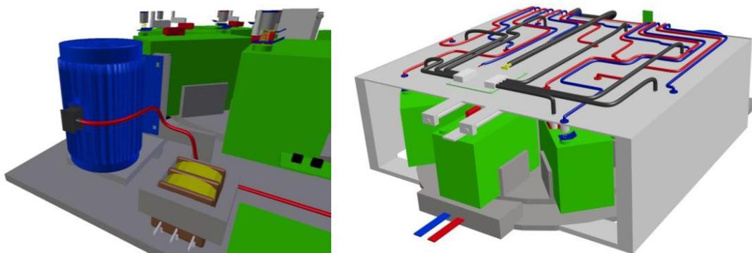
Fig. 11. (a) Possible location of the electric motor, (b) Cables
