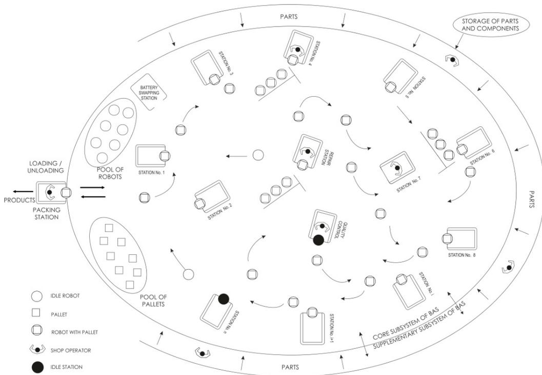
Fig. 1. Position of the battery station in the BAS layout
