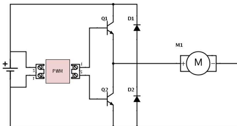
Fig. 10. DC motor controller
