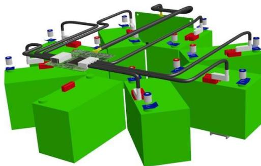
Fig. 9. Data multiplexer of a BMS
