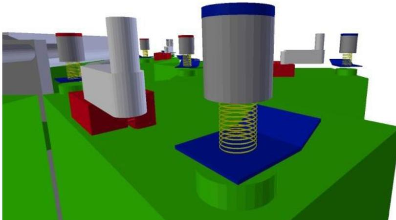
Fig. 4. Contact between battery and charger
