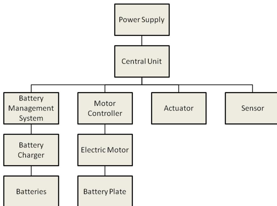
Fig. 2. Block scheme of the battery swapping station
