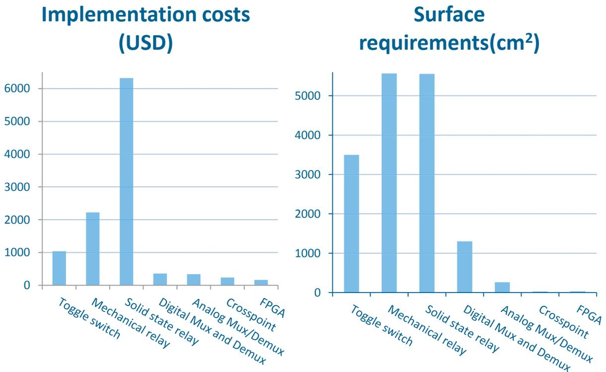
Fig. 2. (a). Implementation costs of various solutions regarding the signal switching matrices;
