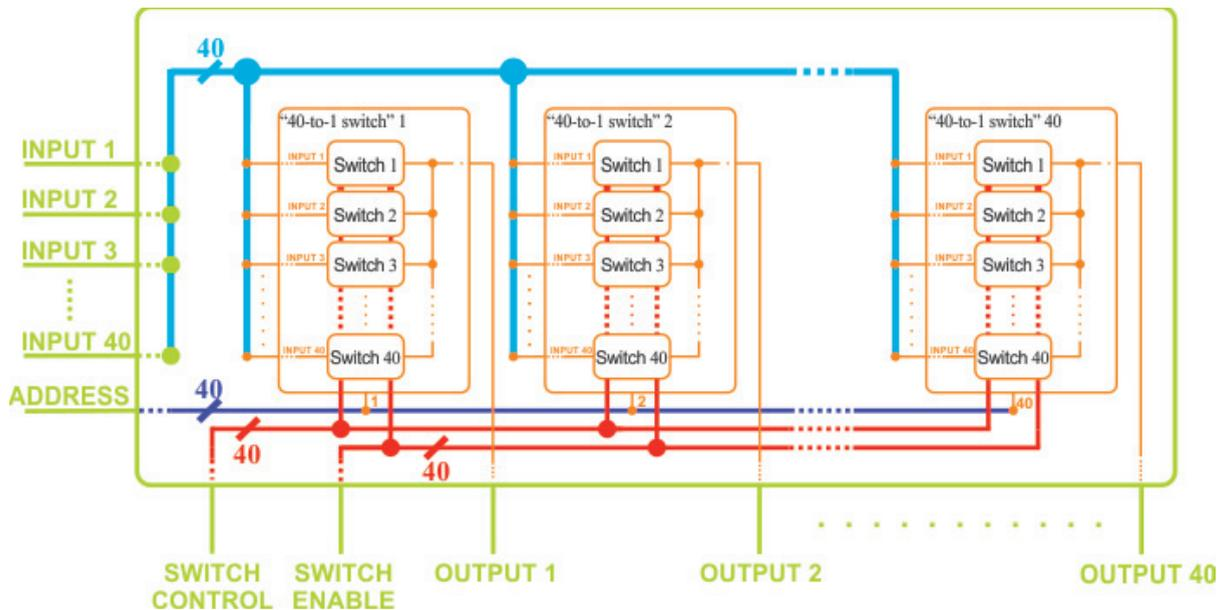
Fig. 1. Implementation of the signal switching matrix using an FPGA device.
