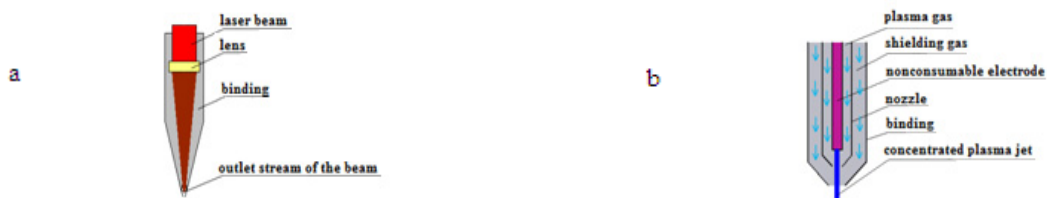
Fig. 2. (a) the principle of operation of the laser nozzle; (b) the principle of operation of the plasma nozzle.
