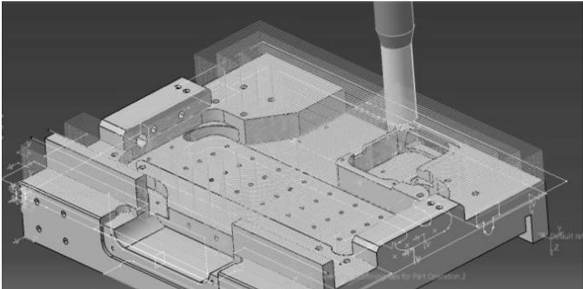
Fig. 1. prismatic milling process on selected CAD component [11].
