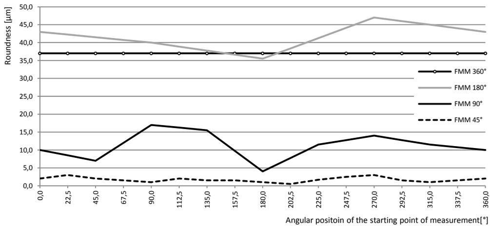
Fig. 4. Roundness of the ring with 3-angular deviation measured with incomplete contour of a circle on the FMM.
