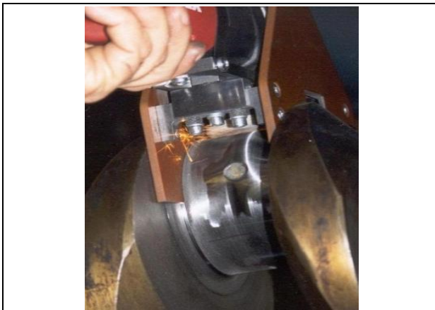
Fig. 5. In-situ crankshafts grinding device: journal with \varnothing 120 mm
