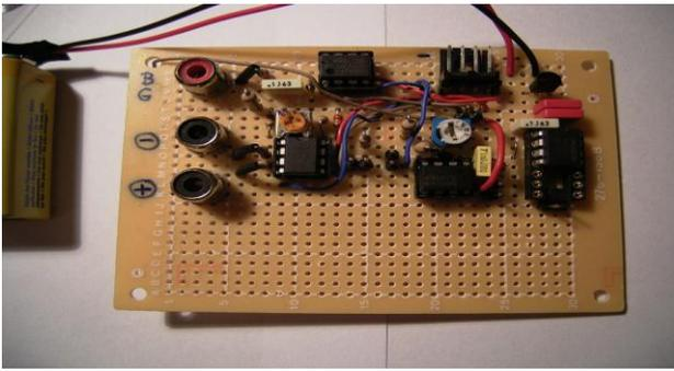
Fig. 4. Signal conditioning board
