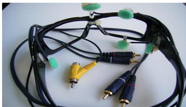
Fig. 3. EOG Goggles and shielded cable
