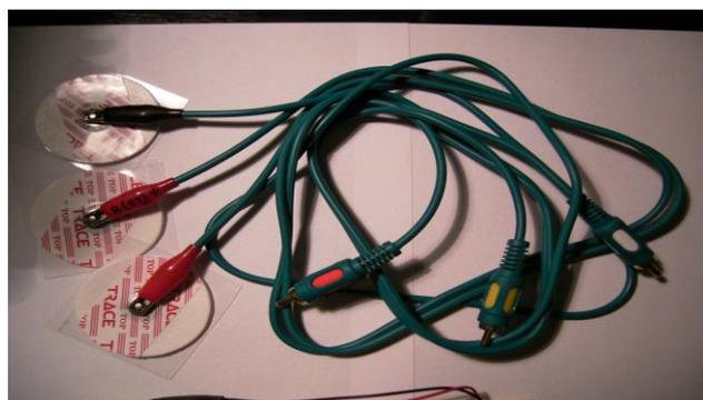
Fig. 2. EKG electrodes and shielded cable
