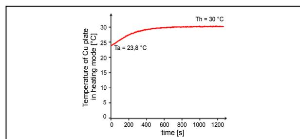
Fig. 2. Characteristic of measured Cu plate to  $T_h = 30^{\circ}C$  by module P1 at ambient temperature  $T_a = 23,8\text{ }^{\circ}C$
