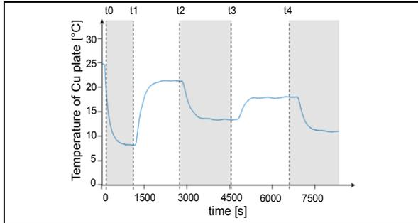
Fig. 3. Temperature of Cu plate cooled by module P2 ( $I_2 = 10A$ ,  $U_2 = 5.5 V$  [P2= 55W]) with change of load P1.
