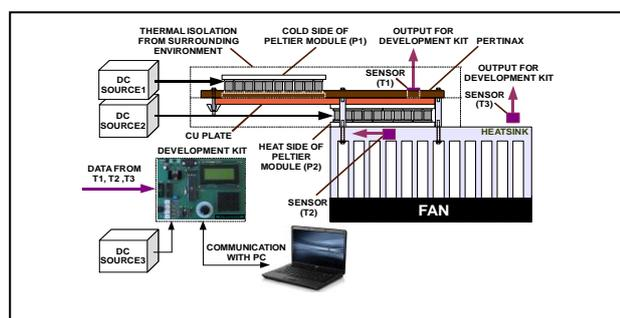
Fig. 1. Equivalent laboratory model of cooling system of trigeneration unit
