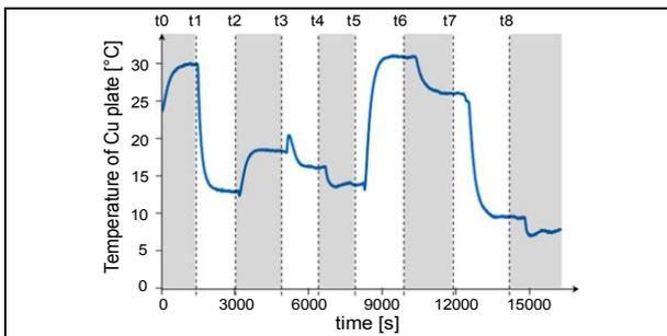
Fig. 4. Temperature of Cu plate with constant load by module P1 and change of cooling power of module P2.
