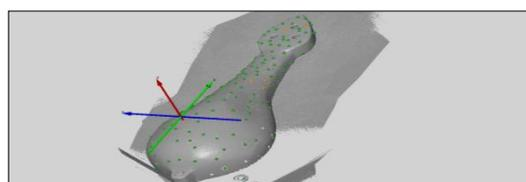
Fig. 3. Common reference points to merge point clouds of different measurement volumes
