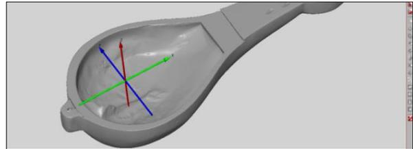
Fig. 8. Completed reverse engineered body of musical instrument
