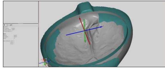
Fig. 7. Completing the inner surface using the CAD cylinder mesh, bridges and surface patches to fill holes and maintaining continuity of point positions and slopes
