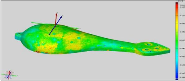
Fig. 4. Surface deviation between different scanning setups after merging of point clouds
