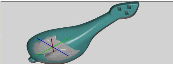
Fig. 6. Inner parts of surface after scanning, cover plate removed from points cloud
