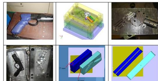
Fig. 3. The tool design, manufacturing and optimising designs of the inserts
