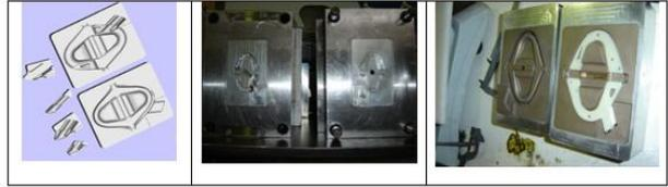
Fig. 4. Design of inserts, Aluminium machined inserts and DMLS produced inserts
