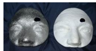
Fig. 4. Thermal-sprayed mask with LS nylon polyamide model
