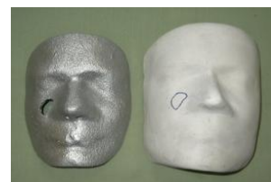
Fig. 2. Thermal-sprayed mask with plaster model
