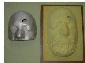
Fig. 3. Thermal-sprayed mask with CNC milled PU model
