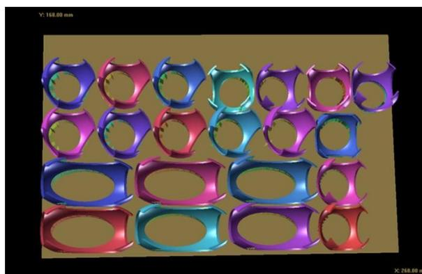
Fig. 2. Visualization of K21 models in scale 1:100 that are prepared for building
