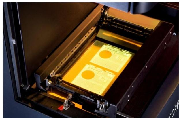
Fig. 1. Building two same parts with ZBuilder Ultra
