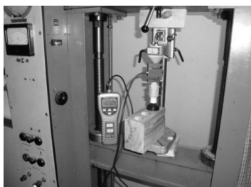
Fig. 4. Force measurement on the testing machine
