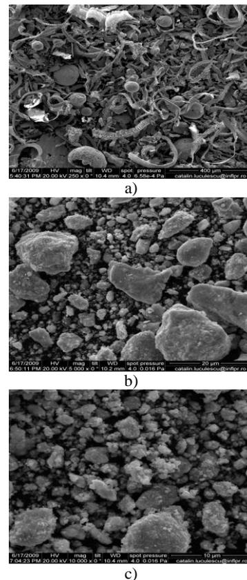
Fig. 1. SEM images of the powders :a) initial powder; b) after 10 hours of milling; c) after 20 hours of milling
