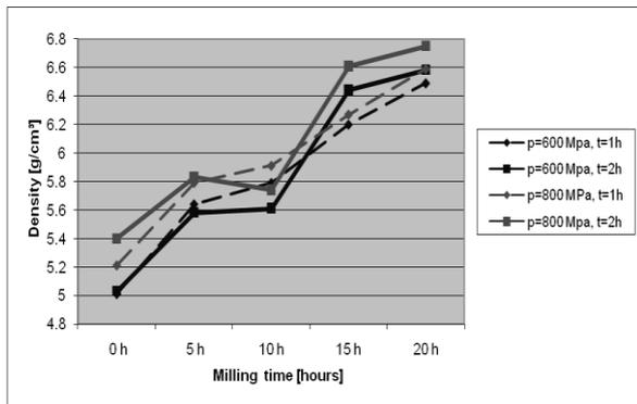
Fig. 4. The densities of sintered parts at 1250 °C
