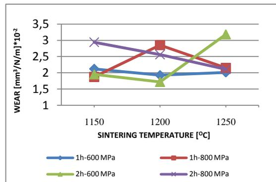
Fig. 7. Evolution of wear function the sintering and compaction parameters
