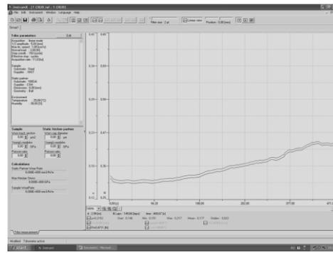
Fig. 6. Friction coefficient of the sample pressed at 800 MPa and sintered at 1250 °C with dwell time of 2 hours
