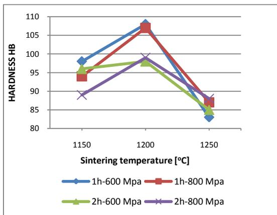
Fig. 5. Evolution of hardness function the sintering parameters
