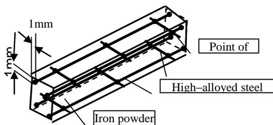
Fig. 1. The emplacement of the steel yarns reticulation inside the sintered iron piece
