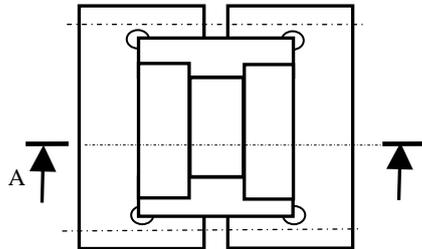
Fig. 2. The mould shape for pressing parallelepipedic samples
