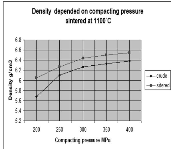
Fig. 5. Density variations of pieces dependent on compacting pressure
