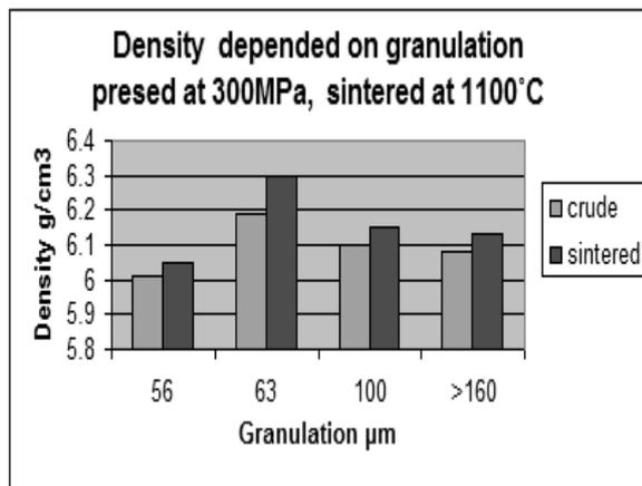
Fig. 4. The pieces density made of powder with different granulation
