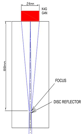
Fig. 1. Ultrasonic beam geometry and specimen with a disc reflector
