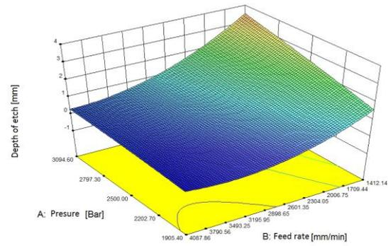
Fig. 3. Variation of depth of etch as a function of feed rate and water pressure using a abrasive rate 0.55 kg/min
