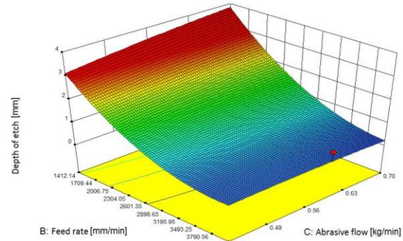
Fig. 4. Variation of depth of etch as a function of feed rate and abrasive flow using a water pressure 3094 Bar
