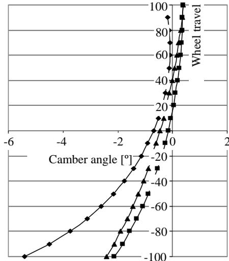
Fig. 4. The wheel camber angle depending on wheel travel (positive for spring compression) in the case of virtual models from fig. 1 (♦), fig. 2 (■) and fig. 3 (▲)
