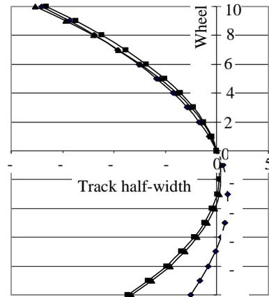
Fig. 5. The track half-width depending on wheel travel (positive for spring compression) in the case of virtual models from fig. 1 (♦), fig. 2 (■) and fig. 3 (▲)
