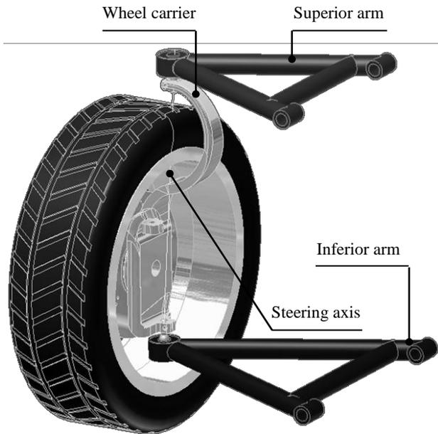
Fig. 3. The virtual model of the suspension mechanism with same ratio of the superposed arms of 0.82 and having superior pivot displaced upward and lateral outward
