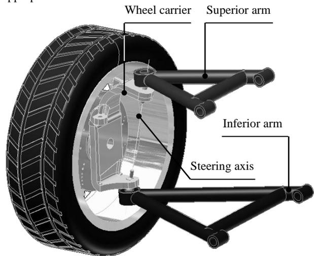
Fig. 1. The virtual model of the suspension mechanism with the ratio of the superposed arms of 0.55
