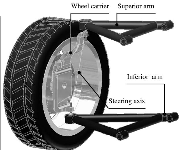
Fig. 2. The virtual model of the suspension mechanism with the ratio of the superposed arms of 0.82
