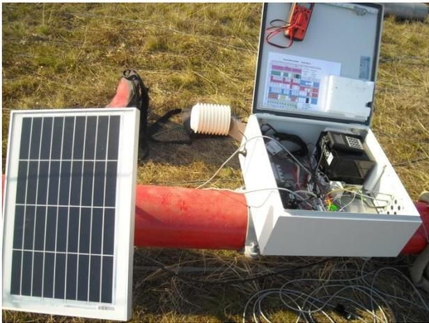
Fig. 1. A photovoltaic panel, a temperature sensor and a steel box containing other auxiliary equipments - all of them attached to the steel pylon
