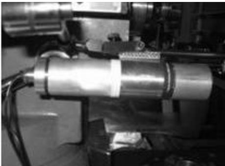
Fig. 1. Diode 2044 mounted on a milling machine
