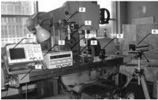
Fig. 4. Test stand for measuring static characteristics of a PSD diode (1-PSD diode with conditioning-power supply circuits in a housing, 2-stabilised laser cooperating with the diode, 3-stabilised power supply NDN DF1731SB5A, 4-two-channel oscilloscope HP 54645A, 5-optical device cooperating with a measurement laser head, 6-laser head of the LSP 30 interferometer, 7-table of a FWD-32J milling machine; 8-magnetic base holding the PSD diode with its PCB, 9-vice for fixing the stabilised laser)
