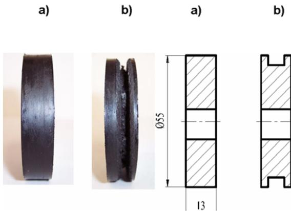
Fig.2. Testing sample for fast wear test
