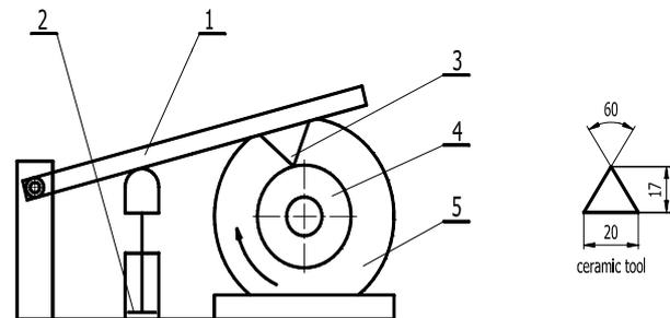
Fig. 1. Design of testing equipment
