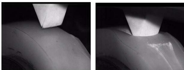
Fig. 3. Ceramic tool during the drop on the testing sample
