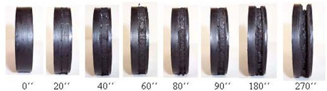
Fig.4. Wear of tested samples in time (0 – 270)s
