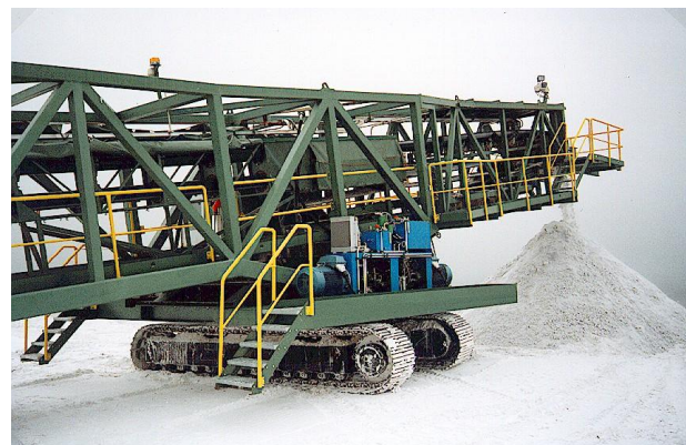
Fig. 2. Variable pipe conveyor
