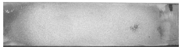
Fig.3. Thermal sprayed piece.
