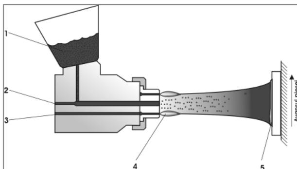
Fig.1. Schematic diagram of the flame thermal spray process and powder. 1-powder, 2-input powder, 3-gas mixture, 4-flame, 5-layer deposited by thermal spray. (Iovănaș, 2006)
