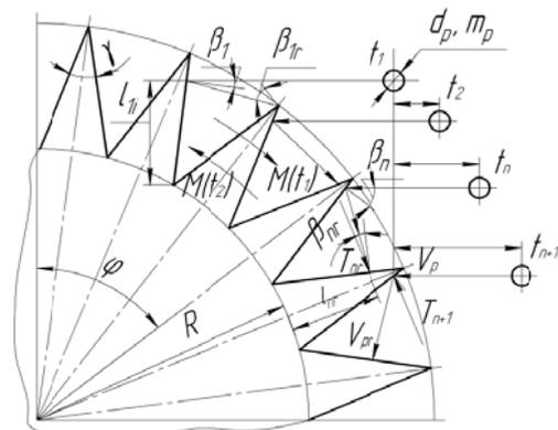
Fig. 1. Design diagram for modeling of the interaction of the abrasive particles flow with part
