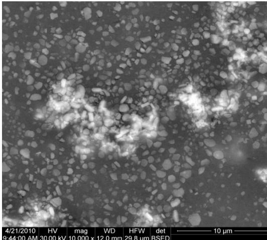
Fig. 1. SEM micrograph of the Al/ $TiB_2$  composite
