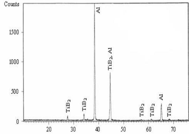
Fig. 3. X-ray diffraction (XRD) pattern of Al/ $TiB_2$  composite
