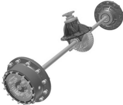
Fig. 2. Motion-transmission system in the Romanian articulated lumber tractor
