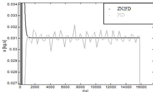
Fig. 3. Comparison of the feeding profiles between ZN2FD and PID controllers
