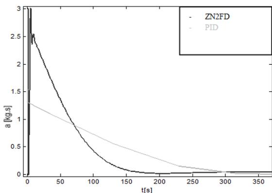
Fig. 2. Comparison of the feeding profiles between ZN2FD and PID controllers at the beginning of the process
