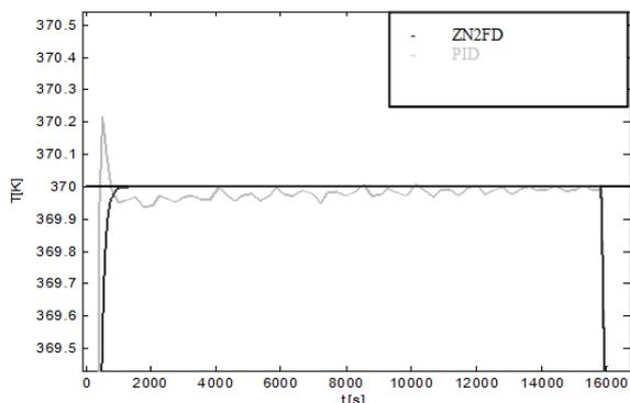
Fig. 1. Comparison of the temperature profiles between ZN2FD and PID controllers
