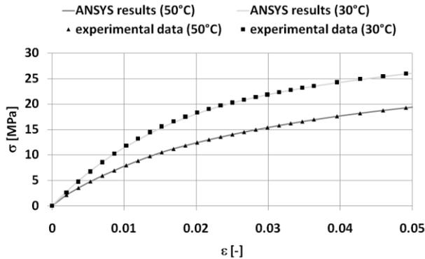
Fig. 3. The comparison of data from experiment and from ANSYS for temperature 30°C and 50°C
