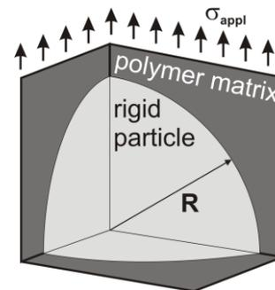
Fig. 2. One eight of the unit cell = FEM model
