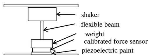
Fig. 2. Test set-up for dynamic measurement
