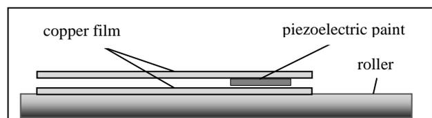
Fig. 1. Piezoelectric paint sensor
