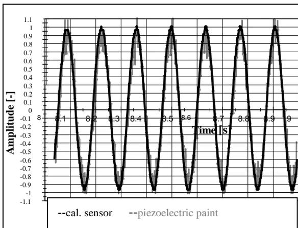
Fig. 4. Correlation between calibrated sensor and piezoelectric paint
