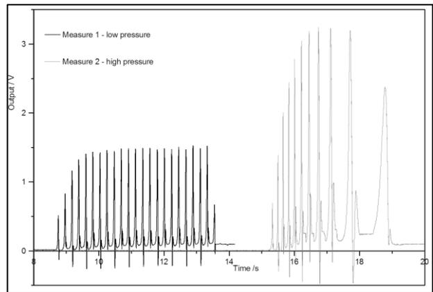
Fig. 5. Piezoelectric paint under elastomer coating– the nip pressure is first increasing and then decreasing
