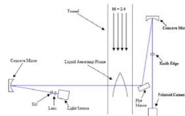
Fig. 2. Schlieren photography setup
