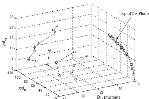
Fig. 4. Liquid aeroramp penetration and droplet distribution
