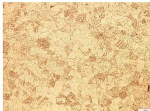
Fig. 3. Microstructural aspect of experimental austenitic stainless steel in solid solution state at 1050°C/ air cooling, (Royal glycerinated water attack, x200)
