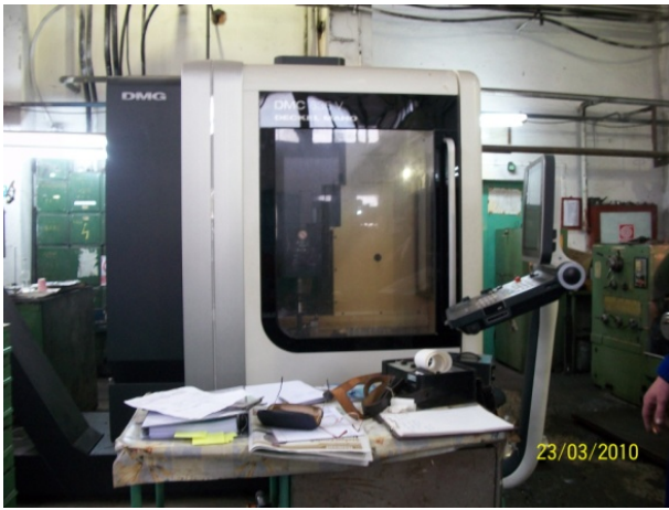
Fig.2. Vertical milling machine DMC 635v
