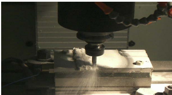
Fig.1. Fiber glass material machined –first test
