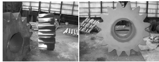
Fig. 5. Gear after machining and sandblast operation
