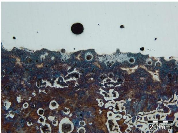
Fig. 2. Microstructure of the bond between 316L and cast iron EN-GJS-700-2
