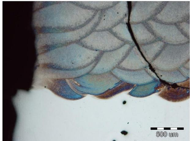
Fig. 3. A crack in the bond between FeCrV15 tool steel and 316L stainless steel
