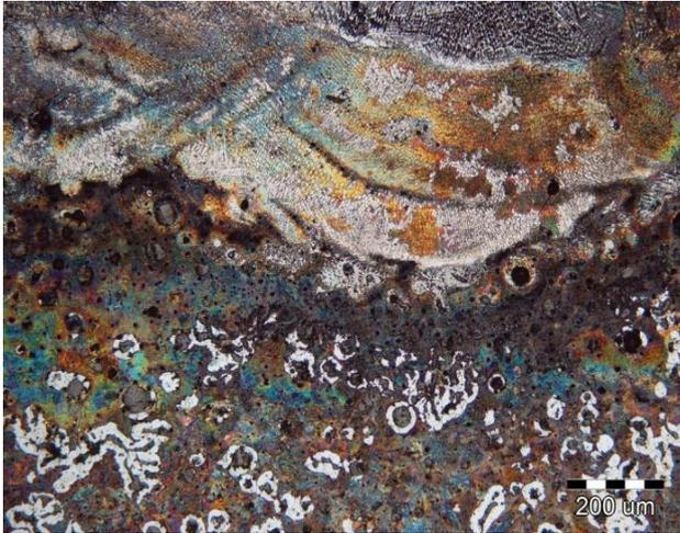
Fig. 1. Microstructure of the bond between AISI H13 tool steel and cast iron EN-GJS-600-3
